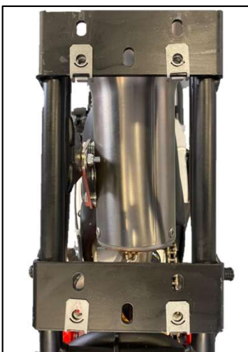
4x Clip (Please, re-use the 2 clips already installed in the rear frame)
