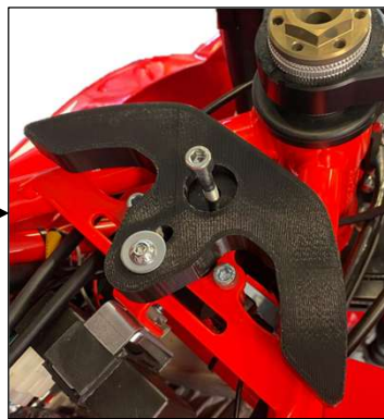
1x M6x35 Screw (to be used to screw the tank cover to the frame) 1x M6x25 Screw 1x Spacer 6.4x18x1.6
