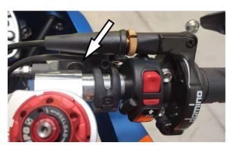
Before each use, check the brake fluid level through the appropriate porthole located on the front and rear brake pump (see pictures).
