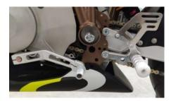
The shift lever is placed On the left side of the engine.
