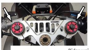
The spring preload can be set by acting on the appropriate adjusters; screwing in to increase the preload or unscrewing to decrease it.
