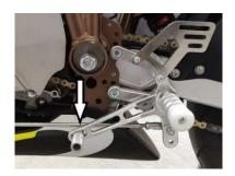
The shift lever is placed on the left side of the engine.
