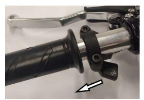
Choke command is placed on the left side half-handlebar for mod. 110 Automatic, 110 4s EVO, 160 4s EVO and GP-2 190 4s.
