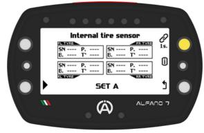
Using the lower and upper left buttons, set the serial number of the sensor you want to associate with the wheel:
