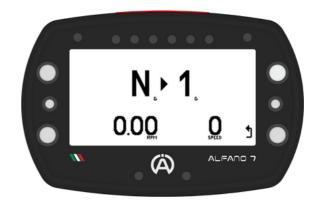
While learning the gear, the gear that the device is configuring is indicated in the center of the screen
