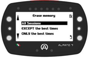
Deleting this data does not remove any tracks you have created, race screens, or any device settings
