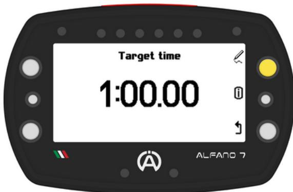
Set the desired time using the upper and lower left buttons.
