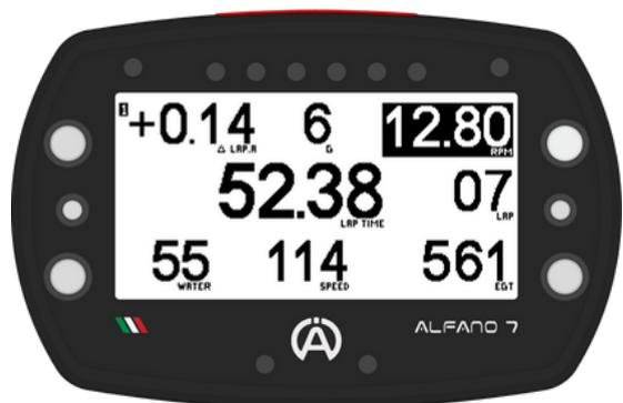
When the device enters race mode, if you have not manually chosen the desired screen in the race screen management menu, the screen used in the previous session will be shown
