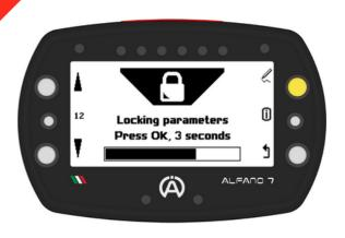
Access to the all settings menu (icon on the bottom left) and access to the Alfano mode selection menu (icon on the centre left) is not possible until the lock is removed
