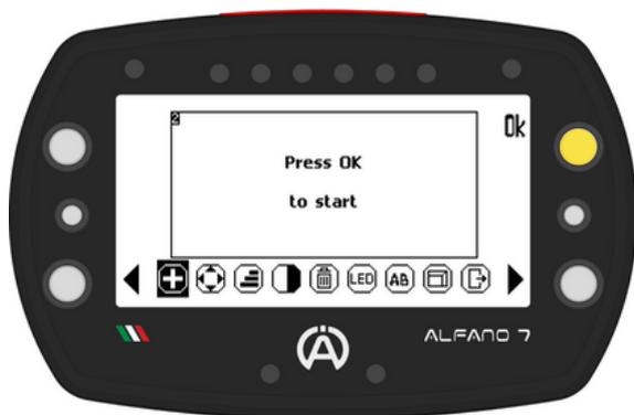
To add a widget clicking "Ok" (when the corresponding icon is selected) a list will open for selecting the desired block
