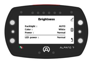
The **9 LEDs** (6 LED system, two alarm LEDs and status LEDs) can also be **adjusted** to **three levels** of **light intensity**: **low**, **normal** and **high**
