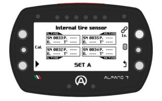
After establishing the connection, you will be able to read the detected air pressure and internal air temperature values
