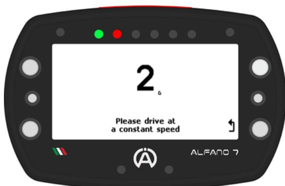
Enter the requested gear and continue learning until the last gear is reached (value entered in the previous screen under the "number of gears" item)
