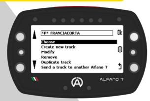
In professional mode the user must select the track in which he wishes to record the data before starting, by opening the "choose" menu all the professional circuits in memory will be displayed
