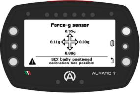
When the Box12 is in the correct position, press the upper left button for one second, corresponding to "1S-CAL", the calibration will be performed
