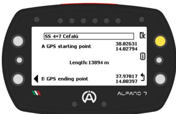
Press 'OK' to save the open track. Pressing the 'back' button will delete the track you just created
