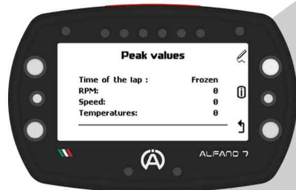
If a **freezing time** is set, when a **maximum/minimum value** is reached on this channel, **Alfabo 7** will **block** the relevant widget (if present on the race screen used) for the set time
