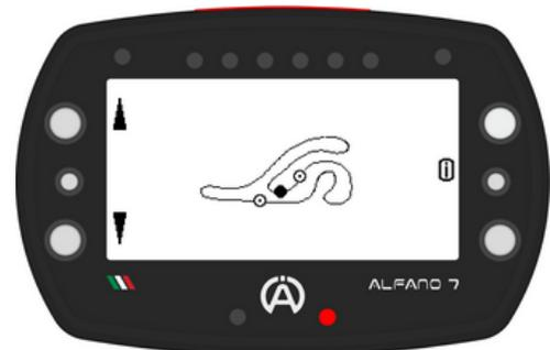
The LED indicator displays a green light if the modified line is at a sufficient distance from the existing lines on the layout, and a red light if it is too close to another line; in this case, it is not possible to exit the modification until the line is in a valid position
