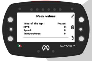
If a freezing time is set, when a maximum/minimum value is reached on this channel, Alfano 7 will block the relevant widget (if present on the race screen used) for the set time
