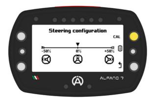
Once the position has been confirmed with the steering wheel fully turned to the left, the cursor will position itself on the 0% value corresponding to a straight steering wheel
