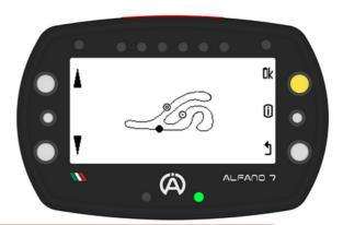
If you do not wish to add any more lines, press "ok" to exit and confirm the positions of the new lines
