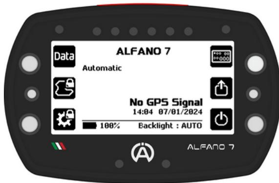
Access to the all settings menu (icon on the bottom left) and access to the **Alfano mode selection** menu (icon on the centre left) is not possible until the lock is removed
