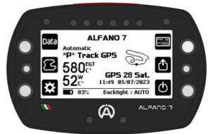
In automatic mode the device works only via GPS for timing the lap and split times (if present on the track in use)
