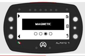
The magnetic mode allows only the use of the magnetic/IR sensor
