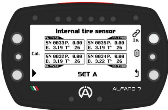
To remove a connected sensor, enter connection mode by pressing the connection button for one second. Then, select the desired internal sensor and press the central left button for one second
