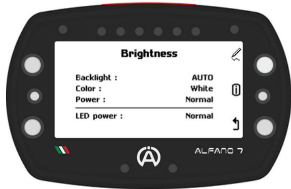
The **9 LEDs** (6 LED system, two alarm LEDs and status LEDs) can also be **adjusted** to **three levels of light intensity**: **low, normal** and **high**
