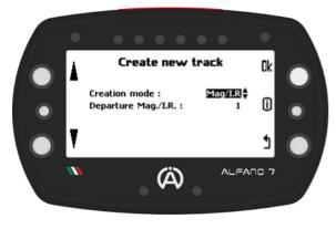
Confirming the "Create new track" item with the "ok" button will open the configuration menu for creating the new circuit if the instrument is receiving the GPS signal
