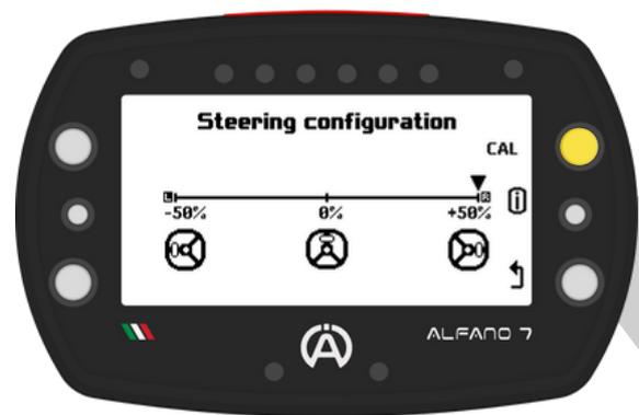
Once calibration is complete, the Alfaano 7 will display the current status of the steering wheel
