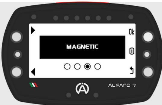
The magnetic mode allows only the use of the magnetic/IR sensor
