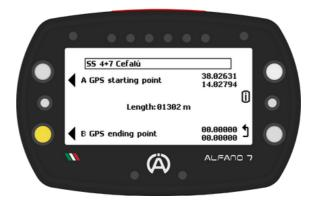
The finish line coordinates will be displayed at the bottom left. You can update the coordinates of point (B) by pressing the corresponding button again (this will update the distance traveled between points A and B)
