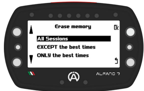
Deleting this data does not remove any tracks you have created, race screens, or any device settings
