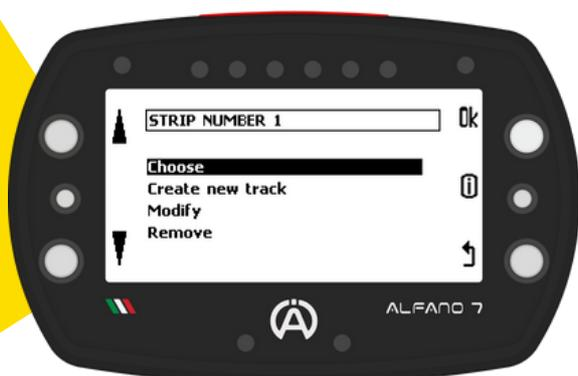
To select a track from memory, open the list of tracks and use the lower and upper left buttons to choose the desired track. Confirm your selection by pressing the 'ok' button
