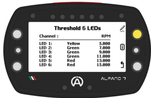
Use the upper and lower left buttons to scroll through the channels. Press the 'ok' button to modify the thresholds and LED color of the selected channel
