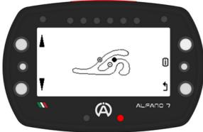
The LED lights up red if the inserted line is too close to a line already present on the track
