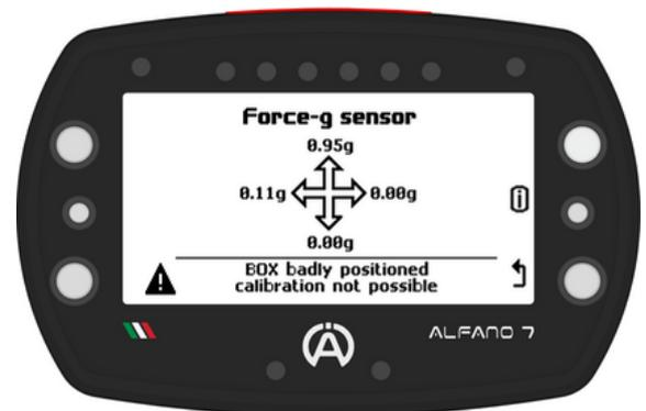
When the **Box12** is in the **correct position**, press the **upper left button** for one second, corresponding to **"1S-CAL"**, the **calibration** will be performed
