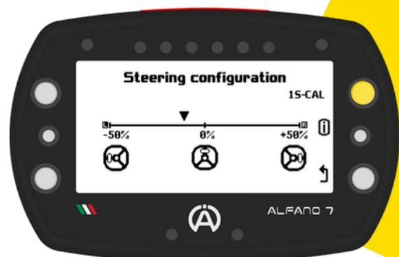
When the start of calibration is confirmed, the cursor is positioned on the -50% value, which corresponds to the steering wheel being turned all the way to the left
