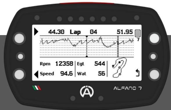
The analysis highlights how the pilot took 44.30 seconds to reach the point under analysis
