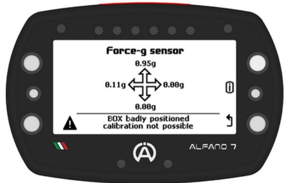
When the Box4Move is in the correct position, press the upper left button for one second, corresponding to "1S-CAL", the calibration will be performed
