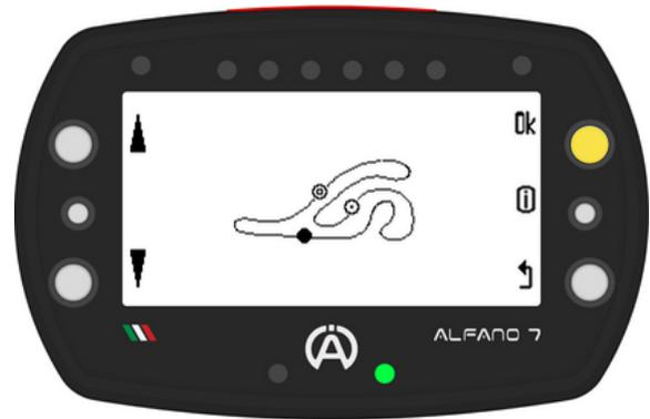
If the device does not allow you to add other lines, you have entered the maximum number of sectors for this circuit or the maximum number of sectors supported by Alfano 7, which is 6
