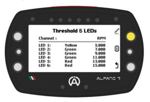
Use the upper and lower left buttons to scroll through the channels. Press the 'ok' button to modify the thresholds and LED color of the selected channel
