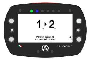
Enter the requested gear and continue learning until the last gear is reached (value entered in the previous screen under the "number of gears" item)
